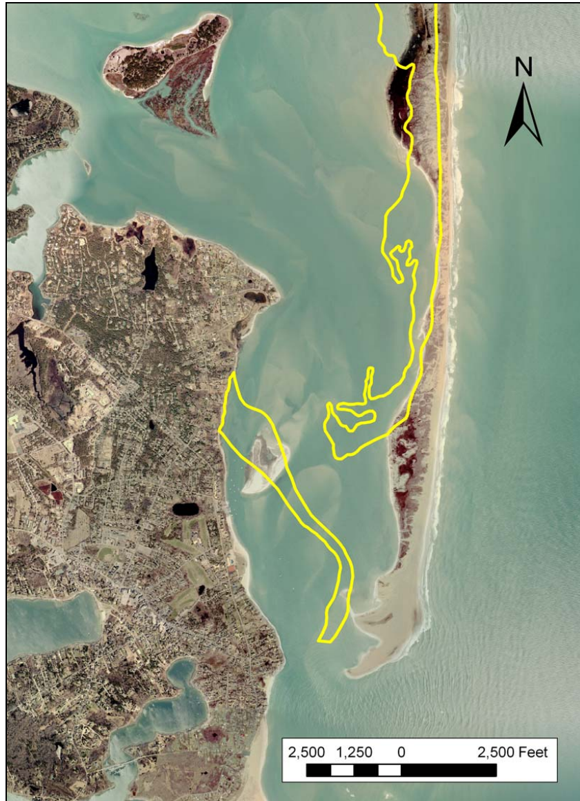
Figure 5. Conceptualization of a single north inlet used for the development of the water quality model run of scenario two.
